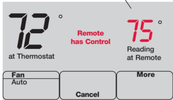
The optional remote control can act as a mobile thermostat, to maintain a comfortable temperature as you move from room to room.
